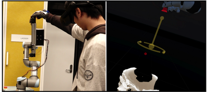
Fig. 18. Robotic arm holding the rotary encoder for rotational interactions according to hand position (left). Select the rotary control in the virtual world and rotate the virtual skeleton around that axis (right).
